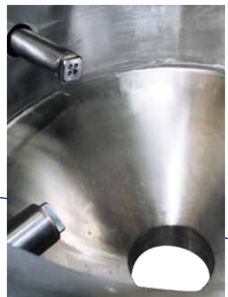
MILLING CHAMBER AND MEGAJET NOZZLES
