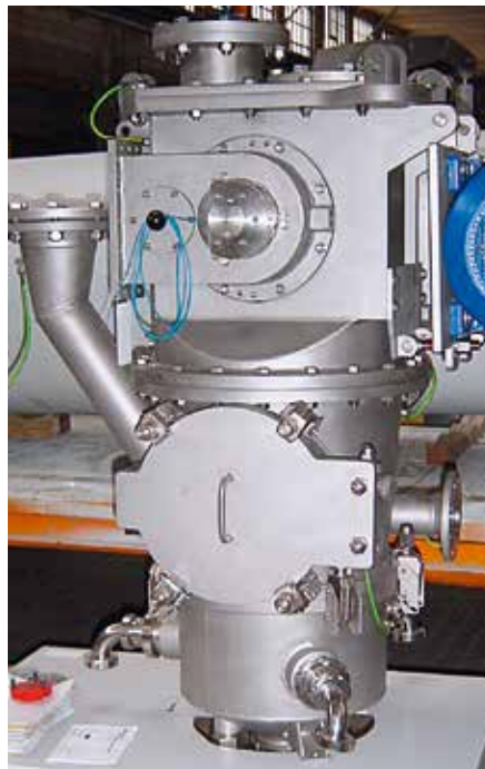
200/400 TTG WITH TURBO TWIN CLASSIFIER HEAD
