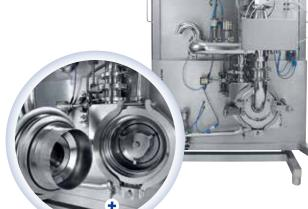
100 UPZ isolator solution with integrated in-line particle analysis and PDD 25 screw feeder
